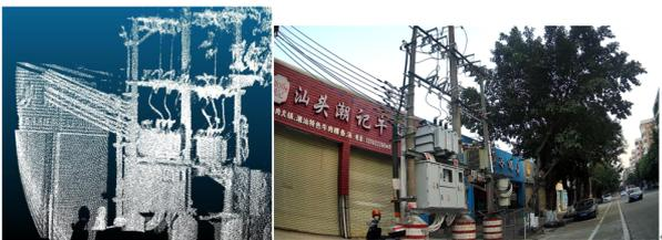
Figure 7. Raw 3D point cloud with visible 2D image
