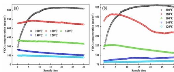
Figure 6. Shows the VOC concentration patterns of modified and reference asphalt under variable temperature heating mode
