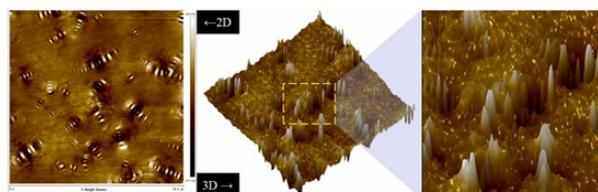
Figure 7. SBS-modified asphalt's AFM morphology
