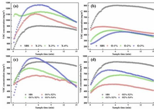
Figure 2. Modified asphalt’s direct smoke suppression performance test results
