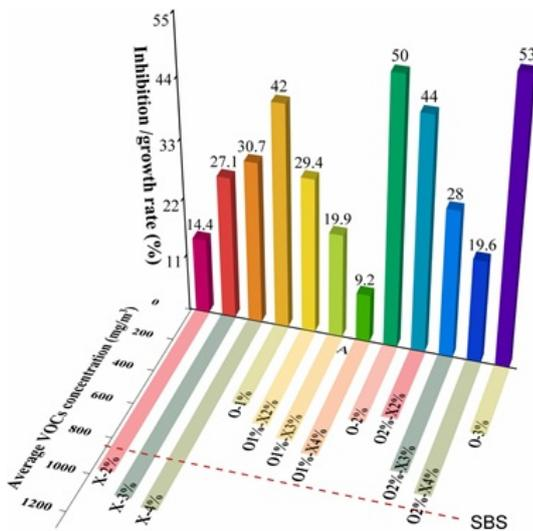
Figure 3. Shows the amended asphalt’s average VOC concentration throughout a 15-minute period
