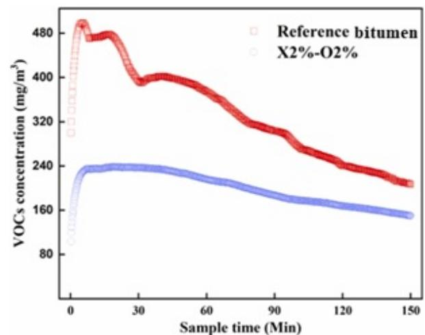
**Figure 5.** Shows the VOC concentration profiles of modified and reference asphalt in heating mode with a constant temperature
