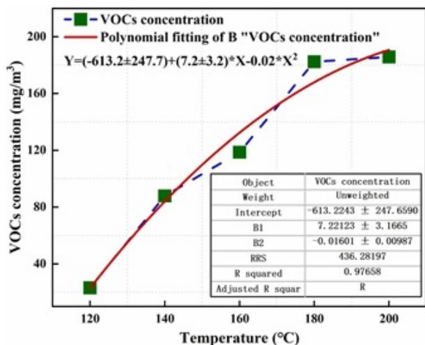
Figure 4. VOC concentration vs. reference asphalt temperature
