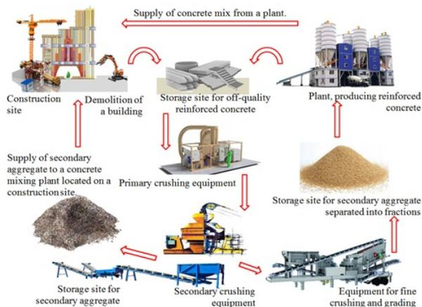
Figure 1. Concrete construction flow chart
