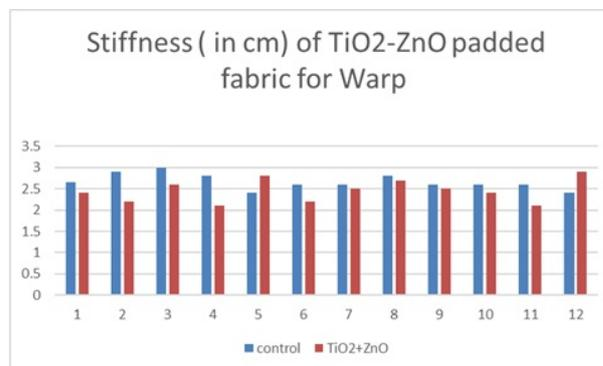
Figure 12. Stiffness of TiO<sub>2</sub>-ZnO padded fabric Warp
